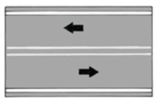
Two-lane, two-way roadway, passing prohibited in both directions, crossing solid lines permitted to turn or in the event of a breakdown.
